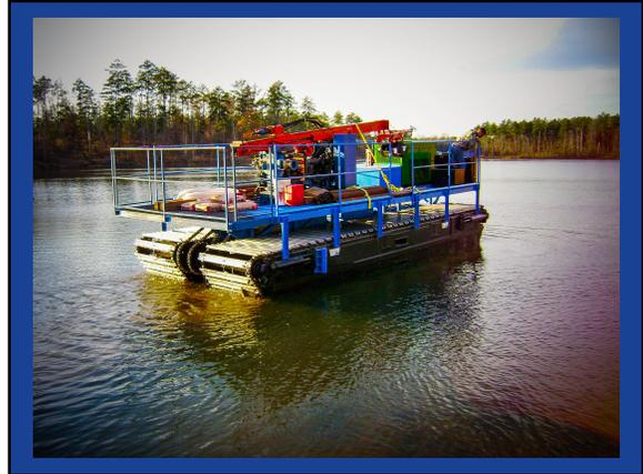
**SPEED:** UP TO 1.5 MPH ON HARD DRY SURFACE & 0.5 MPH IN WATER (2.4 KM/H DRY LAND, 0.8 KM/H WATER)
