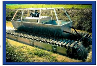
STEERING: STANDARD TRAVEL CONTROLS ONE FOR EACH TRACK IS USED. CAPABLE OF COUNTER ROTATING BY PUSHING ONE LEAVER AND PULLING THE OTHER WITHOUT MOVING BACK AND FORTH OR USING ANOTHER PIECE OF EQUIPMENT FOR ASSISTANCE
