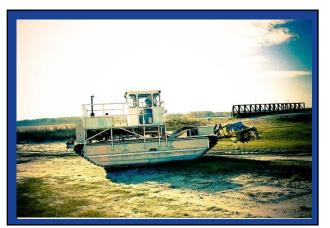
**Steering:** Standard travel controls one for each track is used. Capable of counter rotating by pushing one leaver and pulling the other without moving back and forth or using another piece of equipment for assistance
